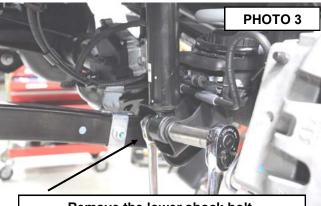
Remove the lower shock bolt.
