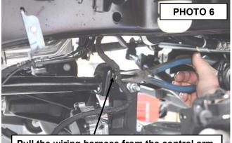
Pull the wiring harness from the control arm.
