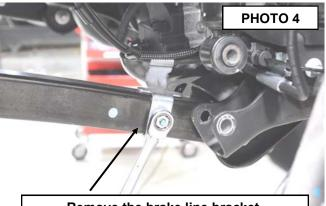
Remove the brake line bracket.
