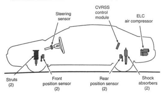
Use a scan tool for diagnosing the electronic suspension. Refer to the scan tool manufacturer's instructions for specific information.
