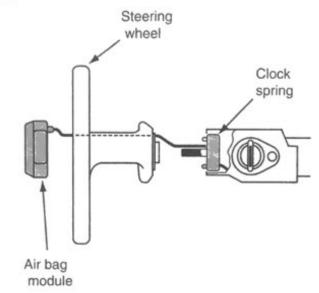
electrical connection as the steering wheel rotates between the inflator module and air bag controller.
