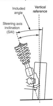
inward tilt of the upper ball joint or strut mount. The angle is measured in degrees from true vertical. If SAI is incorrect, check for a bent component or frame.
