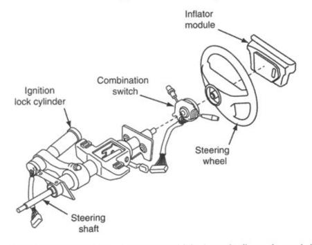
The supplemental inflatable restraint system (air bag) must be disarmed properly before any work is performed on the steering column. Failure to disarm the air bag may result in the accidental deployment of the air bag, which can cause personal injury and unnecessary repairs to the air bag system. Always consult the service manual for recommended procedures on disabling the air bag system.
