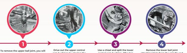
To remove the upper ball joint, you will need a Chrysler ball joint socket. This tool is available from most parts houses and tool dealers. Remember to check which size ball joint you have, because these sockets come in two different sizes. The early models used one size, the later models another. Once you have the proper tool, loosen and remove the upper ball joint.
